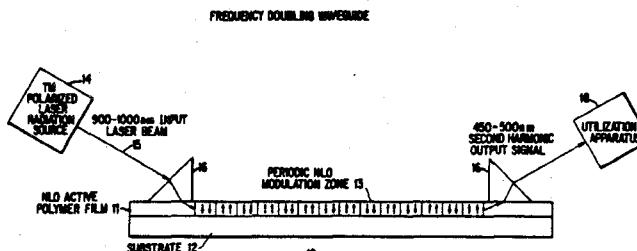
**Optical Waveguide Element, Method of Making the Same, and Optical Coupler Employing Optical Waveguide Element**
